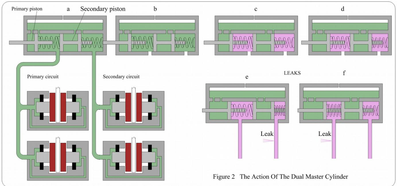
Figure 2 The Action Of The Dual Master Cylinder
