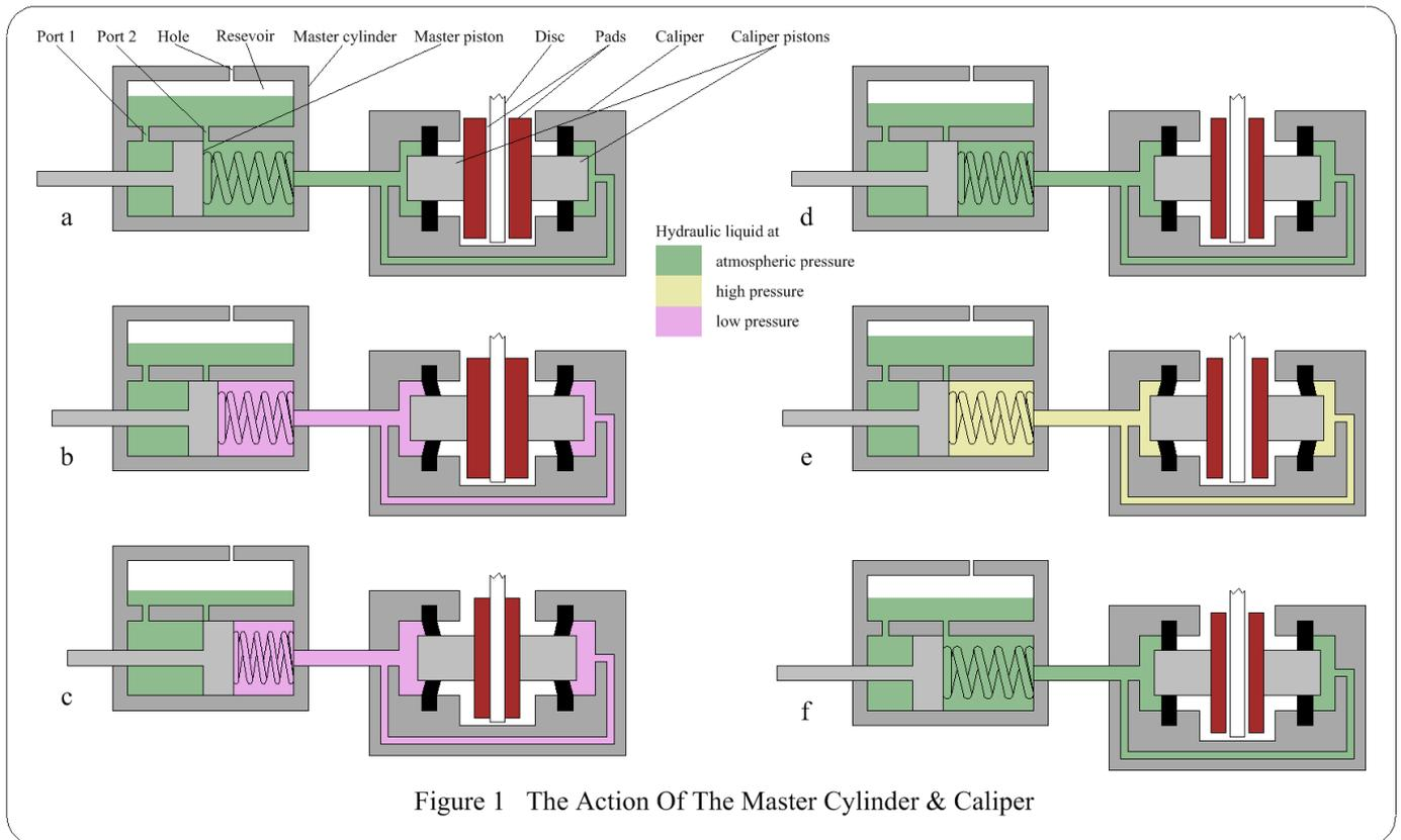
Figure 1 The Action Of The Master Cylinder & Caliper
